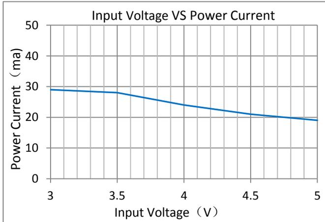
图5: Power Crrnt VS. Suppy Voltage
