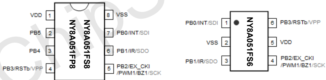
Figure 1 Package pin assignment
