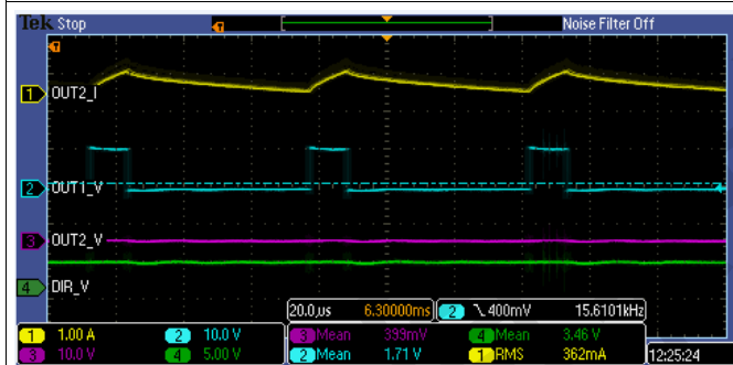
Figure 7. 50% Duty Cycle, Forward Direction
